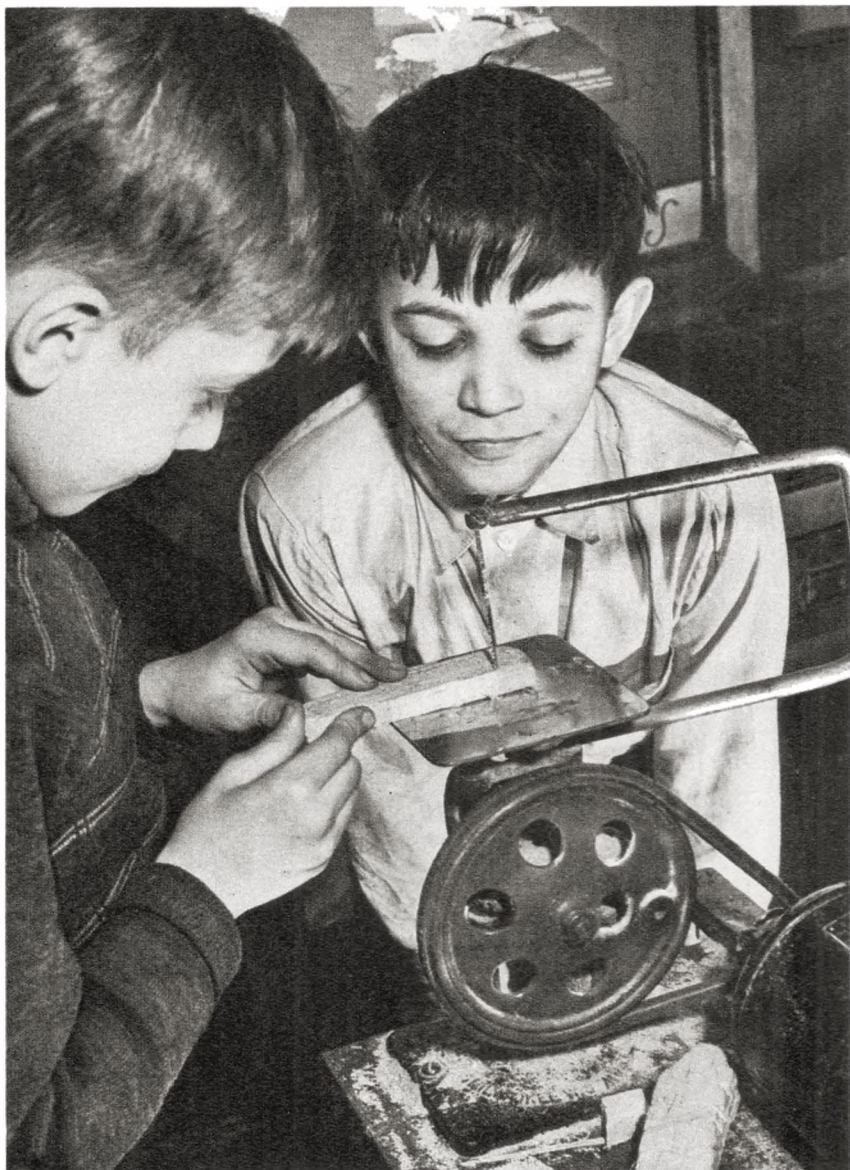
First step in building models is roughing out each plane part with jig saw.
